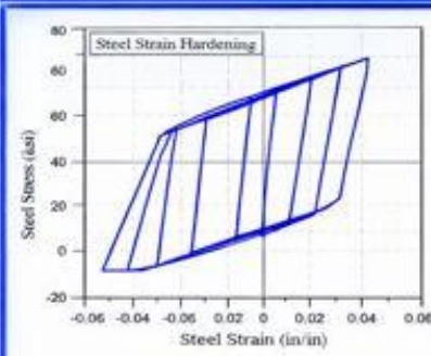
(a) Reinforcing steel model (SH)
